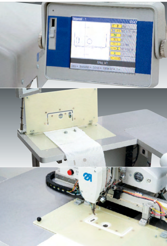
CNC-controlled sewing unit with exchangeable template for overlapped working method – sewing area of max. 380 x 200 mm
